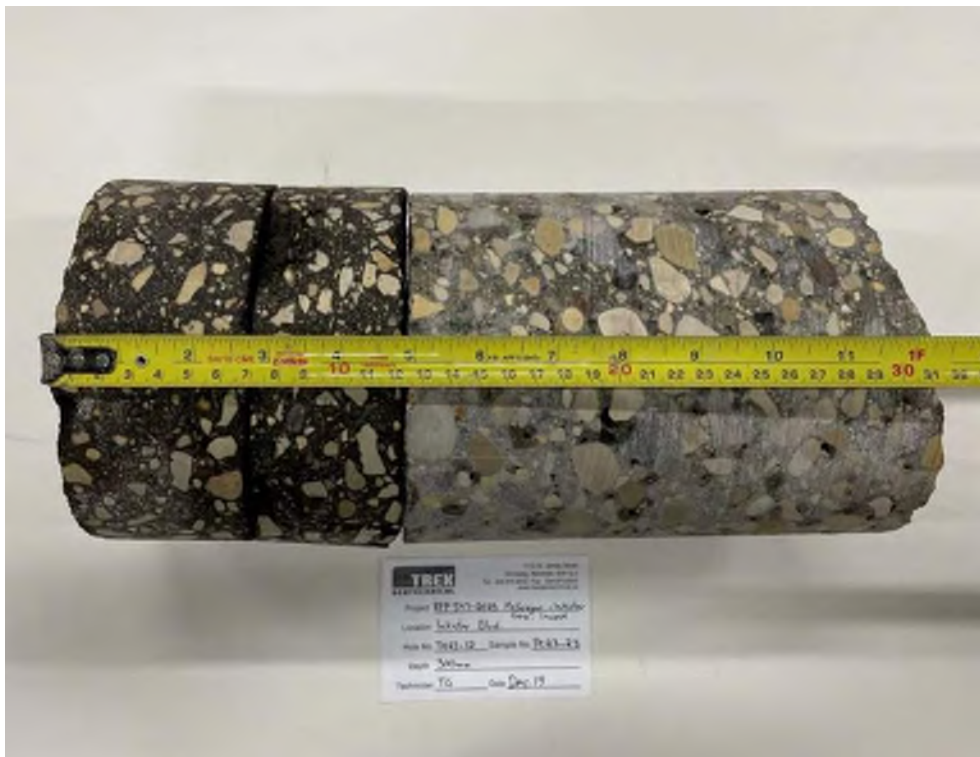
Photo 2: Pavement Core Sample at Test Hole TH23-12
