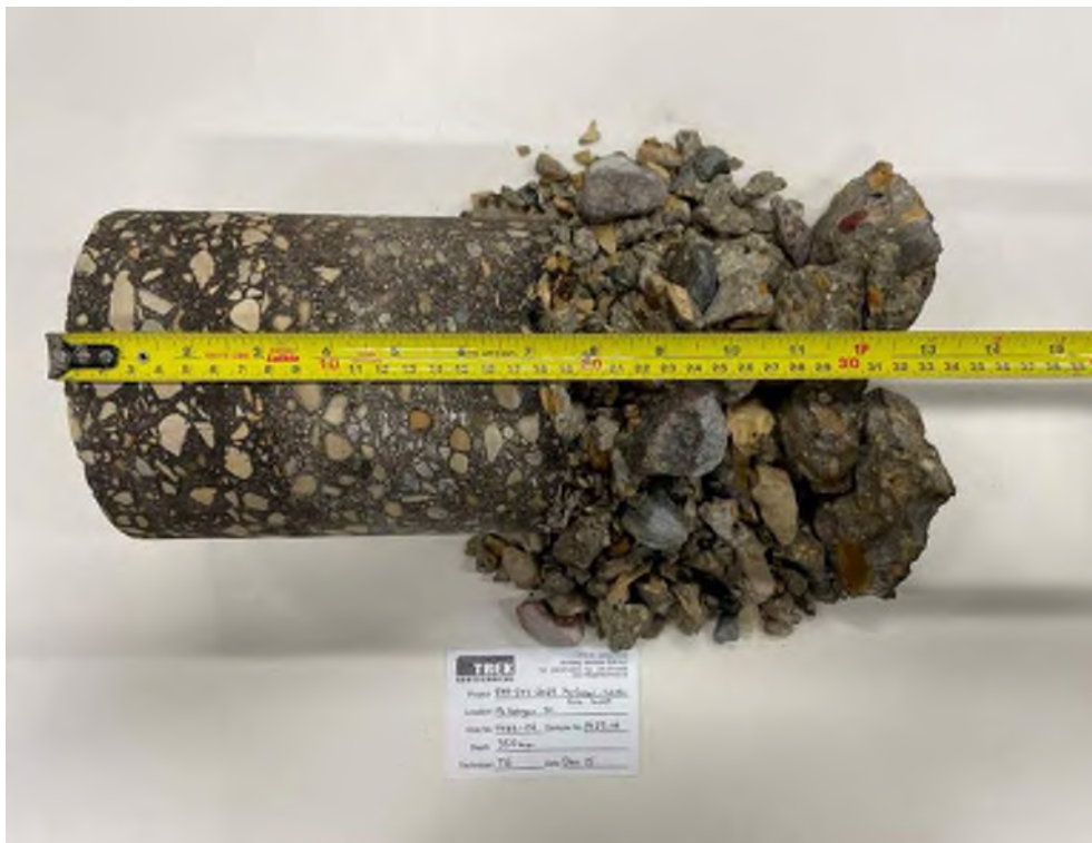
Photo 16: Pavement Core Sample PC23-16
