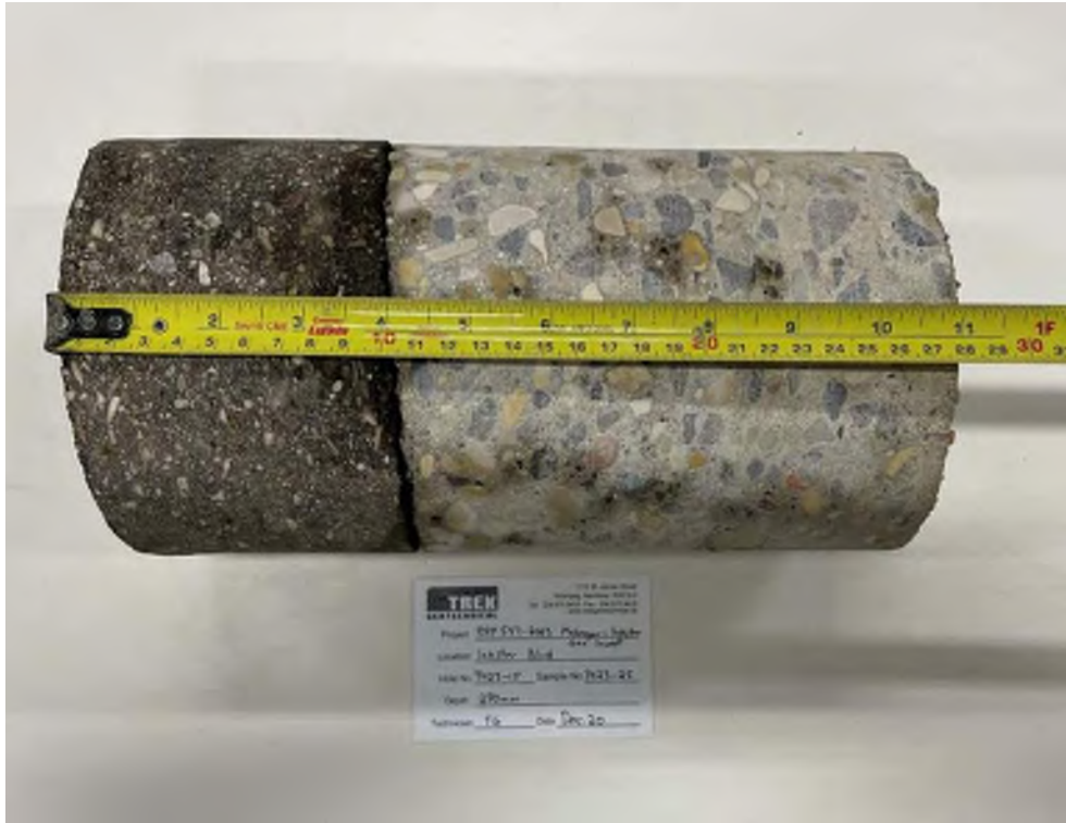
Photo 25: Pavement Core Sample PC23-25
