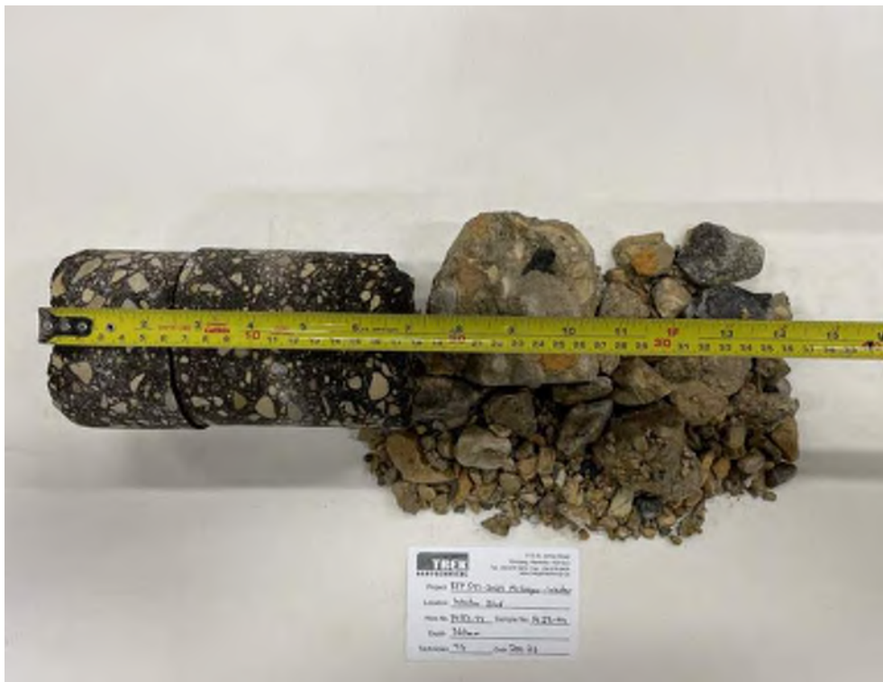
Photo 44: Pavement Core Sample PC23-44
