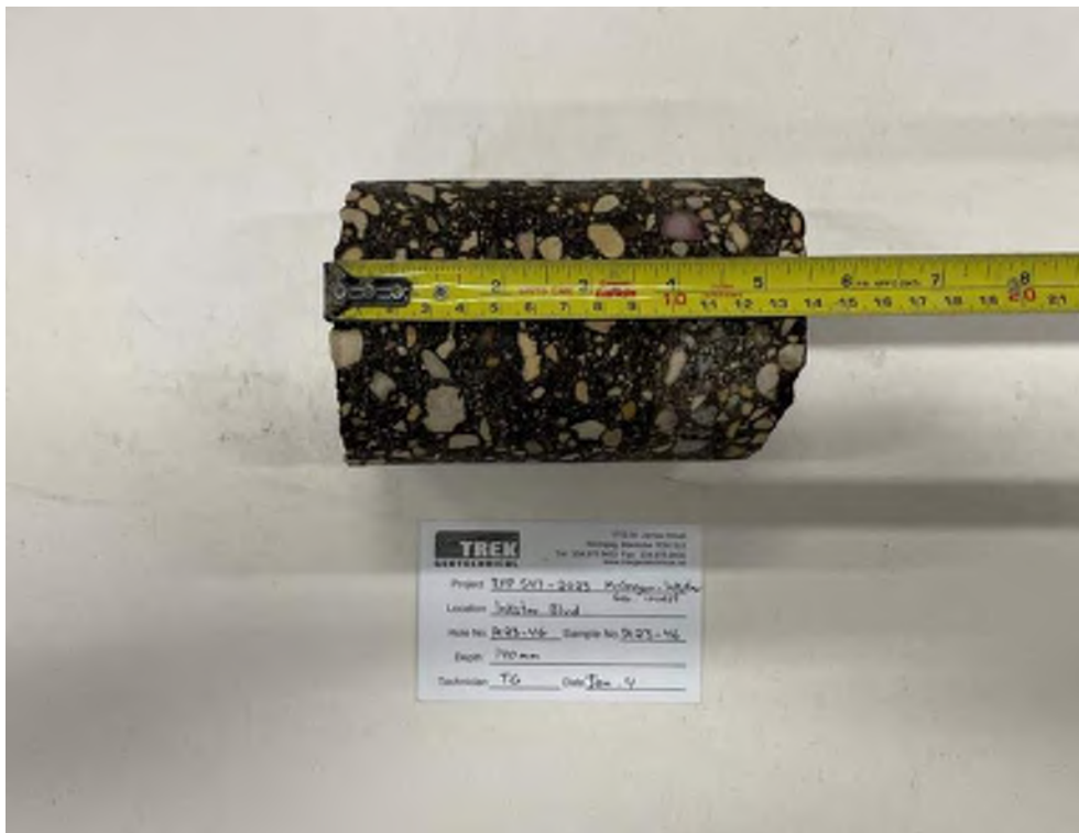
Photo 46: Pavement Core Sample PC23-46
