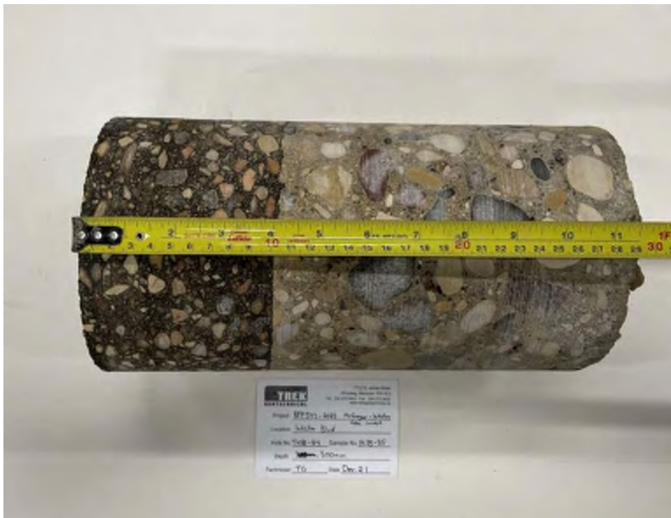
Photo 4: Pavement Core Sample at Test Hole TH23-24
