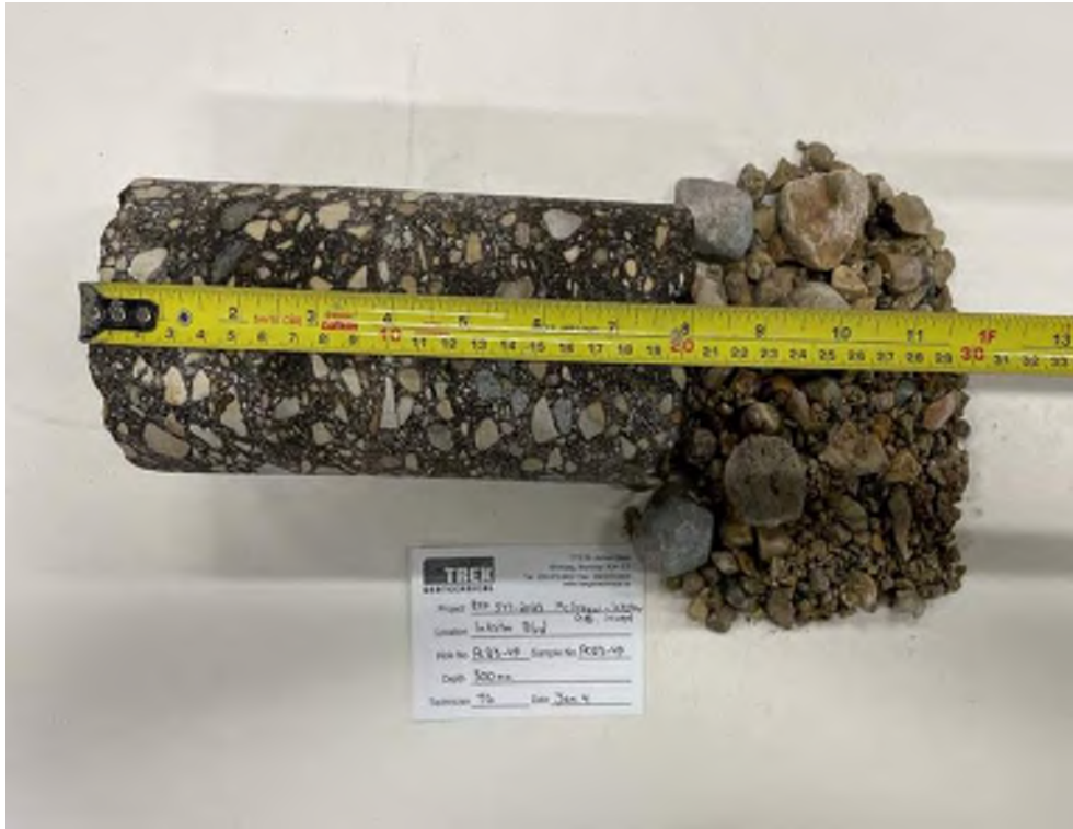
Photo 49: Pavement Core Sample PC23-49
