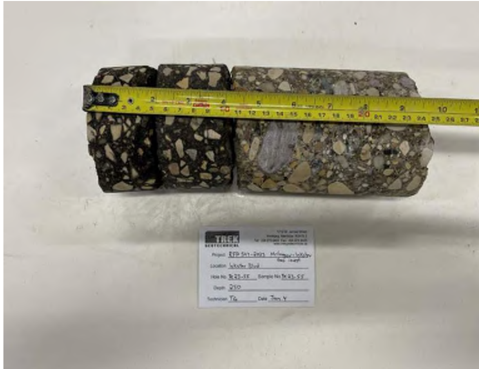
Photo 55: Pavement Core Sample PC23-55
