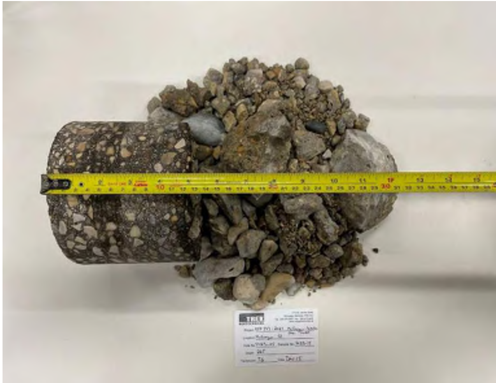
Photo 5: Pavement Core Sample at Test Hole TH23-05
