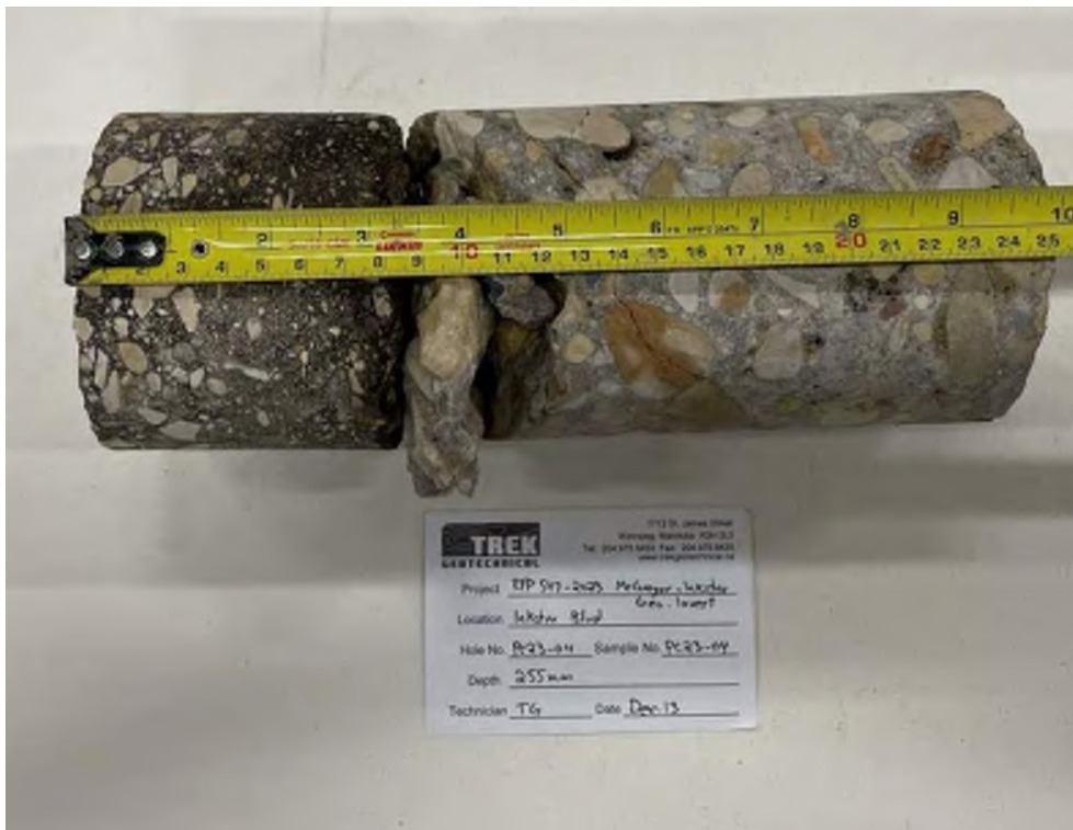
Photo 4: Pavement Core Sample PC23-04
