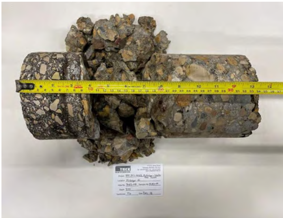
Photo 8: Pavement Core Sample at Test Hole TH23-08
