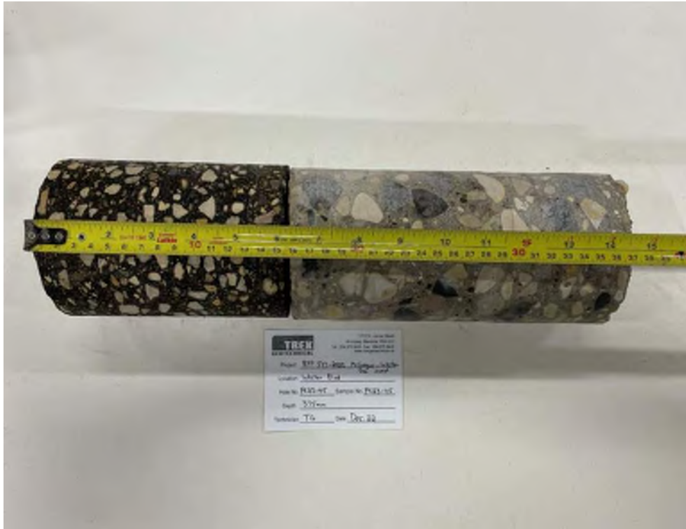
Photo 45: Pavement Core Sample PC23-45
