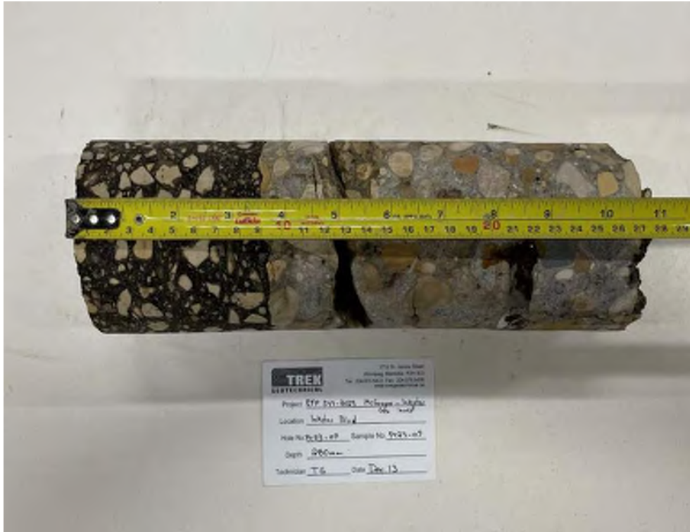
Photo 9: Pavement Core Sample PC23-09
