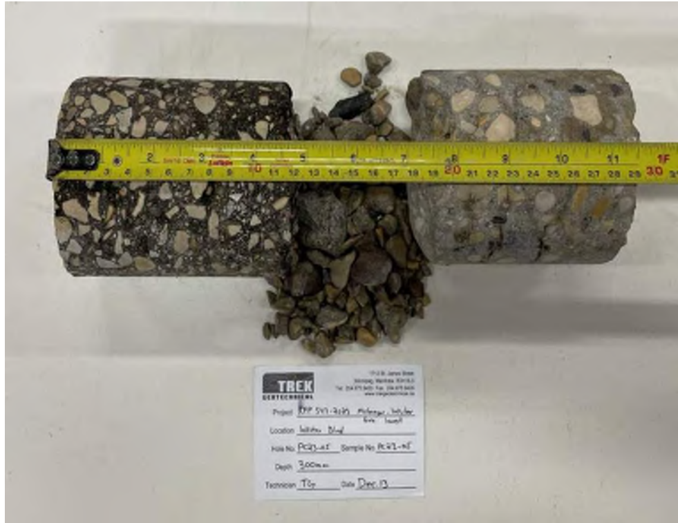
Photo 5: Pavement Core Sample PC23-05
