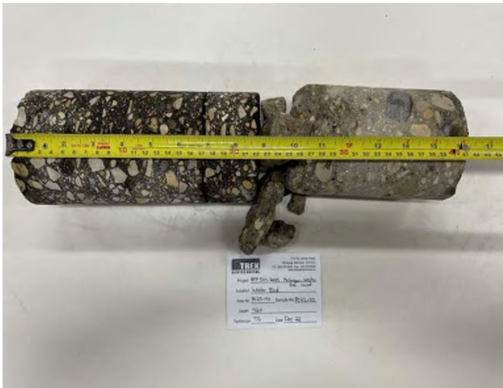
Photo 40: Pavement Core Sample PC23-40
