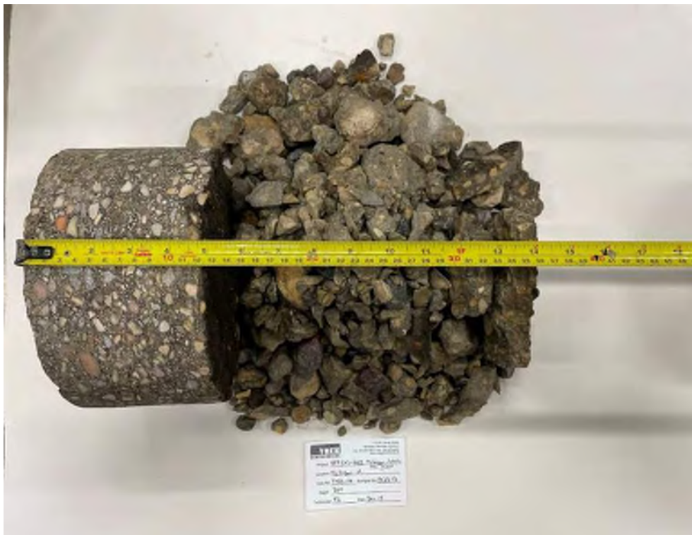
Photo 2: Pavement Core Sample at Test Hole TH23-02
