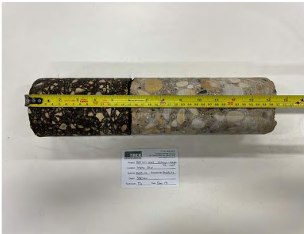
Photo 10: Pavement Core Sample PC23-10
