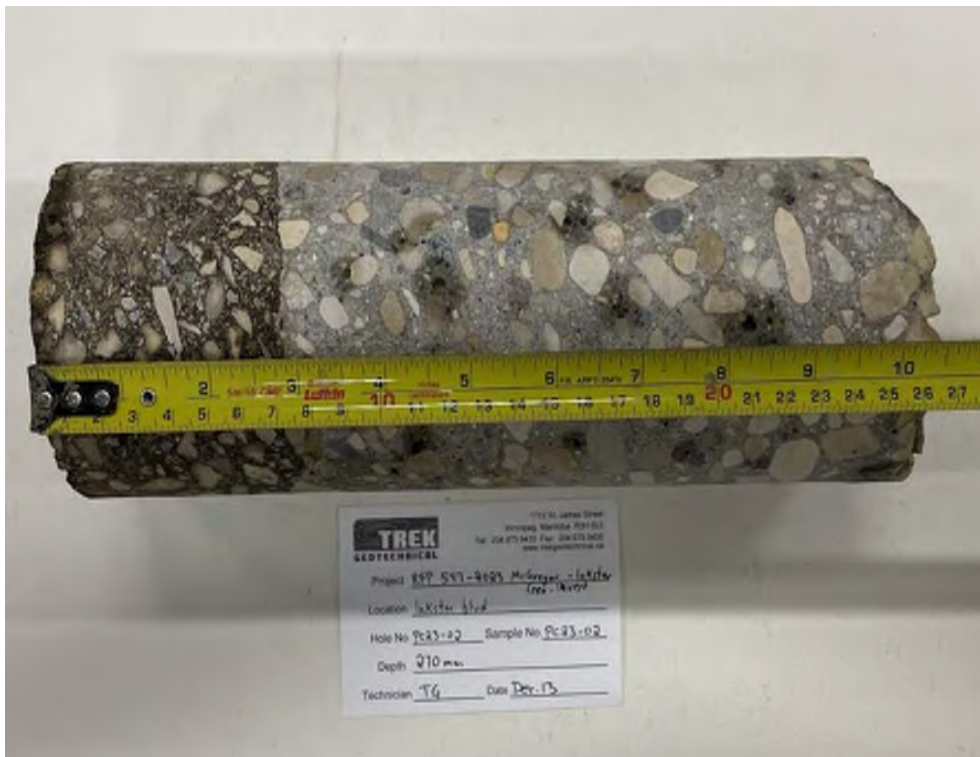
Photo 2: Pavement Core Sample PC23-02
