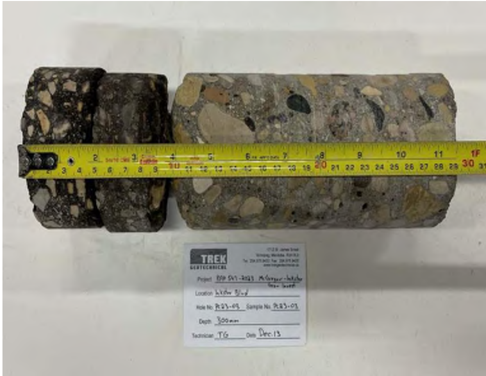
Photo 3: Pavement Core Sample PC23-03
