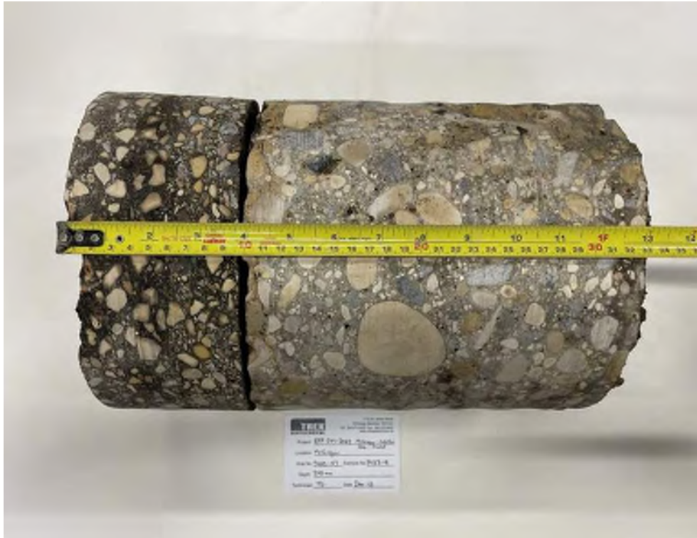
Photo 7: Pavement Core Sample at Test Hole TH23-07
