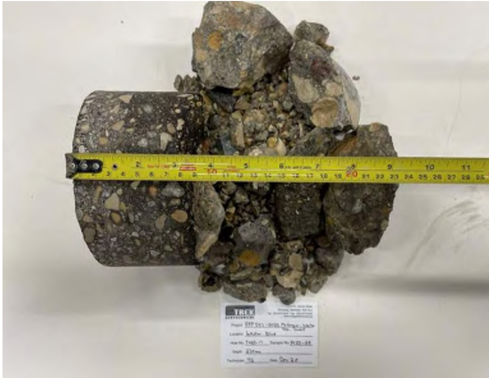
Photo 7: Pavement Core Sample at Test Hole TH23-17
